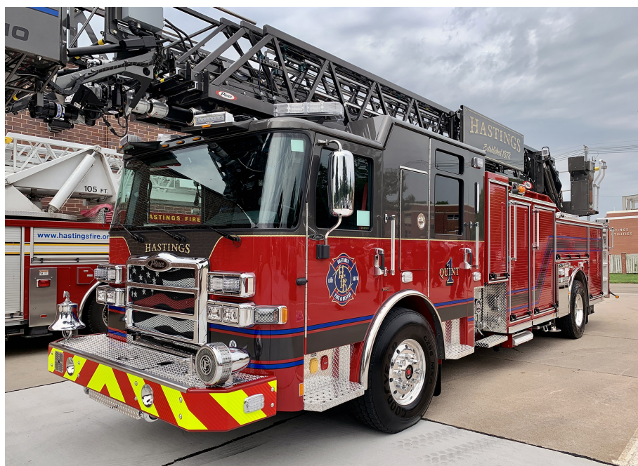
Quint 1 fire apparatus comes with the HFR's tallest aerial device at 110 feet, with the capability to pump 1,500 gallons of water per minute. Photo from City of Hastings Fire and Rescue.
